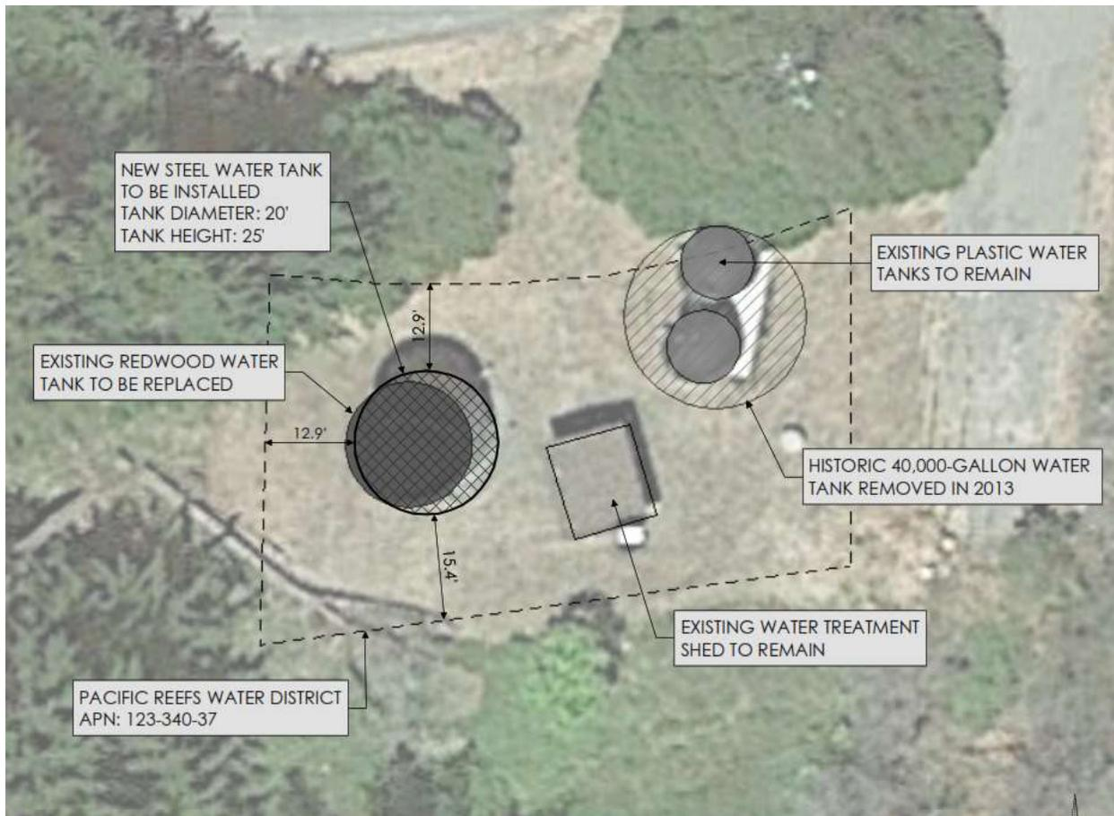
**Figure 3-2: New 30,000-gallon bolted steel water tank replacement project schematic**
