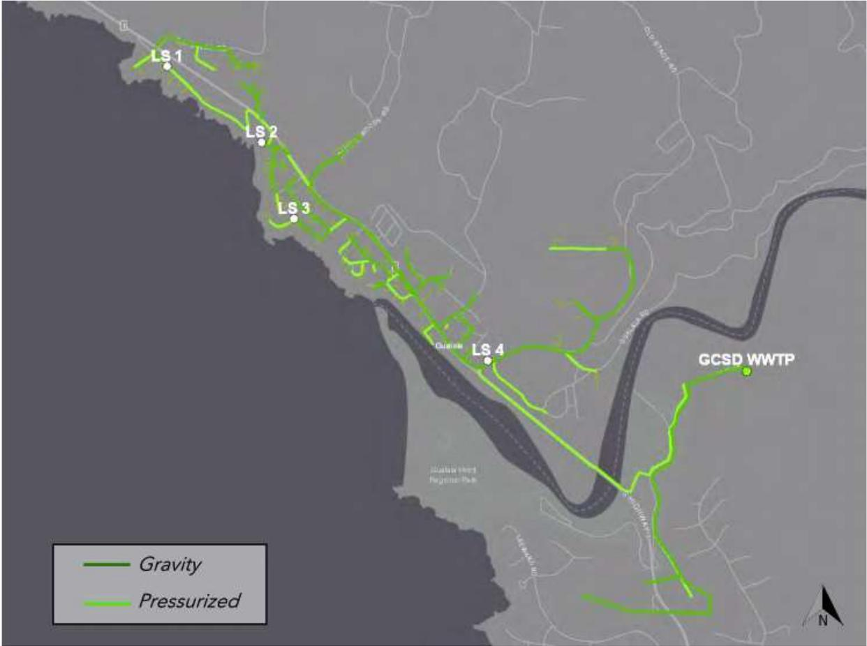
Figure 3-4: GCS D Gravity and Pressurized Sewer Mains
